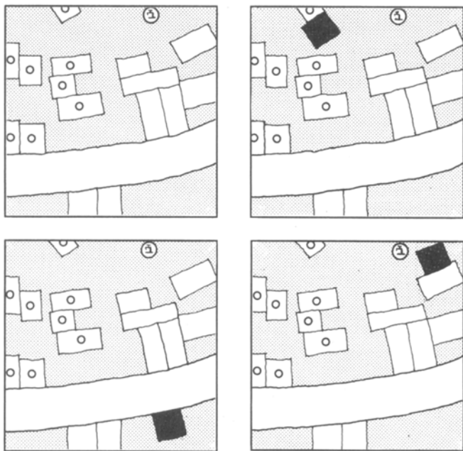
Fig. 15. Self-selection of plots. It is important to have an open plot-allocation system. In informal housing, families can select, according to their particular preferences, the location of their plots within the settlement. Under the self-selection design process, families will be free to choose the location of their plot.
